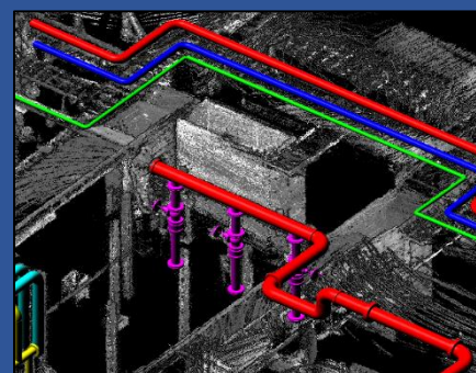
Checking pipeline interference
